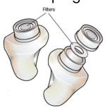
supplying local audiologists and hearing clinics. They can come in filtered or vented/tuned varieties. This means each plug is bored out and then either fitted with an adjustable vent or capped with a button sized filter attached to its outer end.
